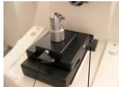
Clamping lever of the trimming block Clamping lever of the trimming adapter
